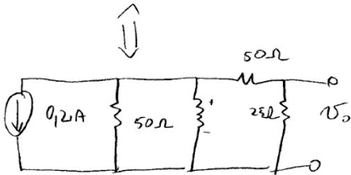
LCK  $0,2 + \frac{v_L}{50} + i_L + \frac{v_o}{25} = 0 \quad ; \quad v_o = \frac{25}{25+50} \cdot v_L$
