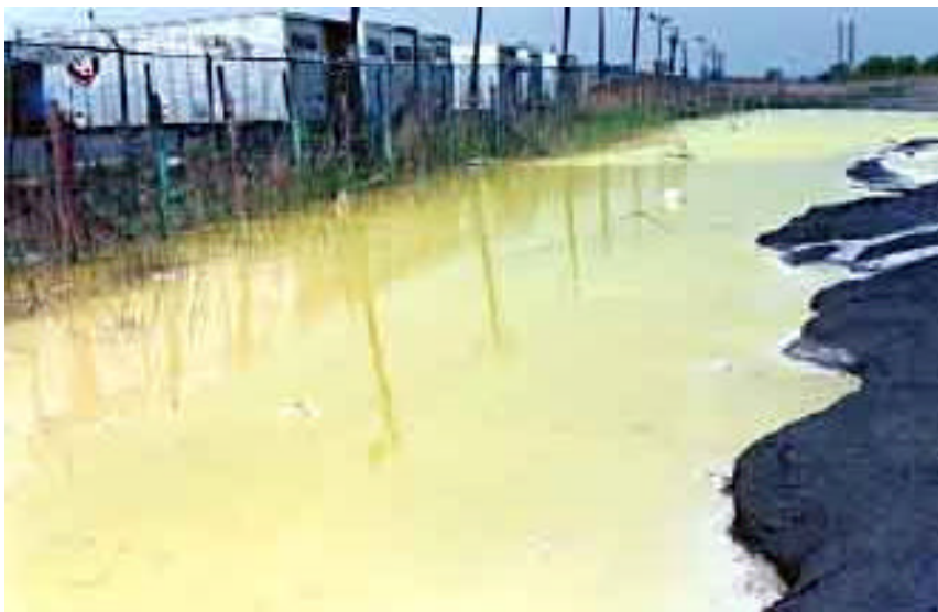
The alchemy of contamination. Chromium in the soil of this New Jersey industrial parking lot has dissolved in a pool of standing water. Because chromium can go into solution and move through soil, chromium pools and blooms (the crystallized chromium left on the surface when the water evaporates) may occur some distance from the original site of contamination.
