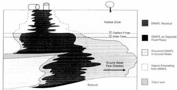
FIGURE 2-5 Conceptual diagram of DNAPL migration through the subsurface. As the diagram indicates, some DNAPL remains as an entrapped residual in the soils (indicated by the dark shading), some migrates as a separate fluid phase (indicated by the black areas), some dissolves in the ground water to create plumes (indicated by the light shading), and some vaporizes into the gas in the soil pores (indicated by white areas).
