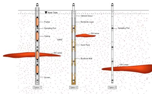
Figure 4. Options for multilevel systems installed in overburden.
