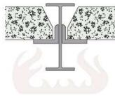
Figure 39 Shelf angle floor beam.
