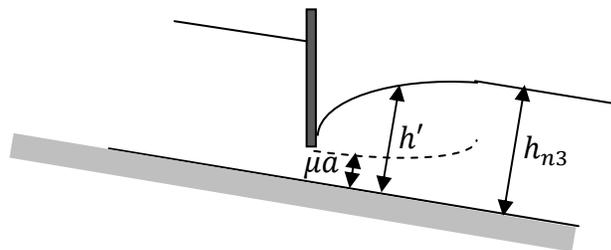
$$m_{h_{n3}} = m_{\mu a + h'} = \frac{q^2}{g(\mu a)} + \frac{h'^2}{2} \rightarrow h' = 0.60 \text{ m} \quad (2.12)$$
