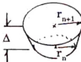
$$V_{\text{Tronco de Cono}} = \pi \cdot \left[ \frac{r_n + r_{n+1}}{2} \right]^2 \cdot \Delta.$$
