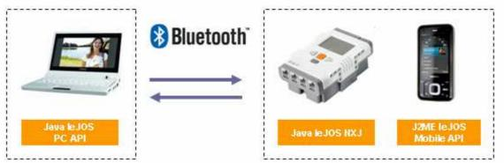
With this kind of solution you can develop your control system in a machine with better resources, for example a PC and send/receive information from your NXT brick but in case of your communication link is broken, the sides, PC and NXT can execute a reconnection routines to stablish the communication again. <u>This idea is really important for complex project in robotics because imagine if you don't add logic in a mars robot for example.</u>
