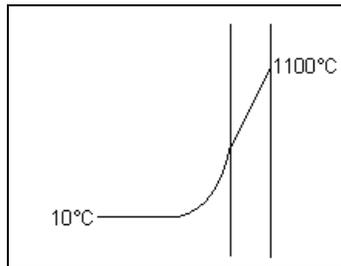
$$q = \frac{A \cdot (T_{h,wall} - T_c)}{\frac{1}{h} + \frac{\Delta x}{k}} = \frac{16 \text{ m}^2 \cdot (1100 \text{ }^\circ\text{C} - 10 \text{ }^\circ\text{C})}{\frac{1}{12 \text{ w / m}^2\text{ }^\circ\text{C}} + \frac{0,1\text{m}}{2,3 \text{ w / mK}}} = 137527 \text{ [w]}$$
