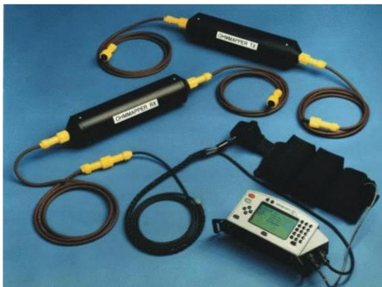
Figura 28: ohmmapper: consola, receptor, transmisor y cables electrodos
