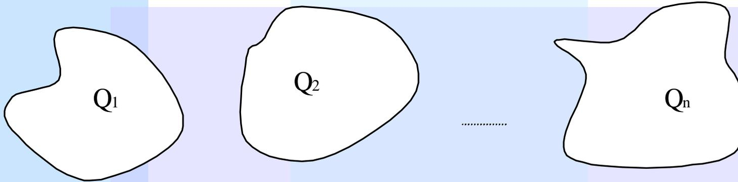
$$W = \frac{1}{2} V_1 \underbrace{\iint_{S_1} \sigma_1(\vec{r}) dS}_{Q_1} + \frac{1}{2} V_2 \underbrace{\iint_{S_2} \sigma_2(\vec{r}) dS}_{Q_2} + \dots + \frac{1}{2} V_n \underbrace{\iint_{S_n} \sigma_n(\vec{r}) dS}_{Q_n}$$
