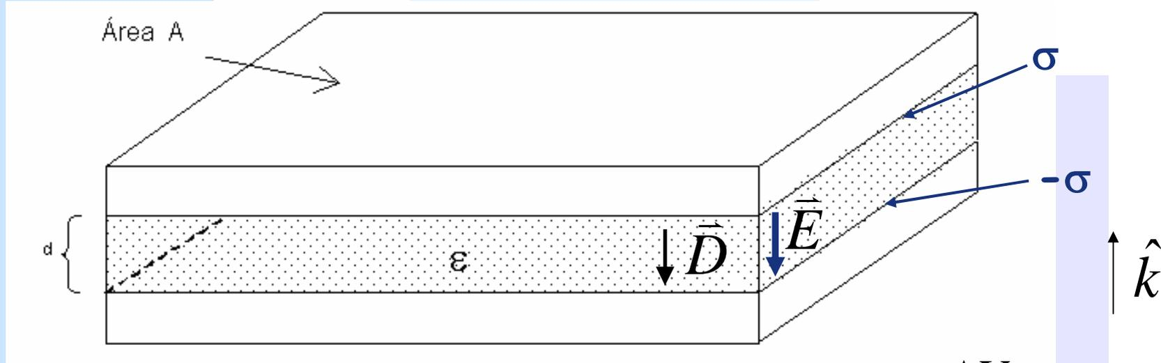
$$\vec{D} = -\sigma \hat{k} \Rightarrow \vec{E} = -\frac{\sigma}{\epsilon} \hat{k} \Rightarrow -\int_{-d}^0 \vec{E} \cdot d\vec{l} = V_{\sigma} - V_{-\sigma} \Rightarrow \overbrace{V_{\sigma} - V_{-\sigma}}^{\Delta V} = \frac{\sigma}{\epsilon} d$$
