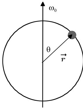
$$\vec{N} - mg\hat{k} = m(2\omega_0\hat{k} \times \vec{v} + \omega_0\hat{k} \times (\omega_0\hat{k} \times \vec{r}) + \vec{a})$$
