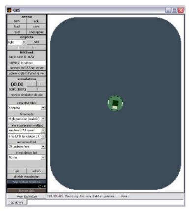
You can move the simulated robot by placing the mouse pointer over the black square on the robot, pressing and holding the left mouse button, and moving the mouse. To rotate a simulated robot, simply repeat this procedure but over any of the dark green areas on the robot.
