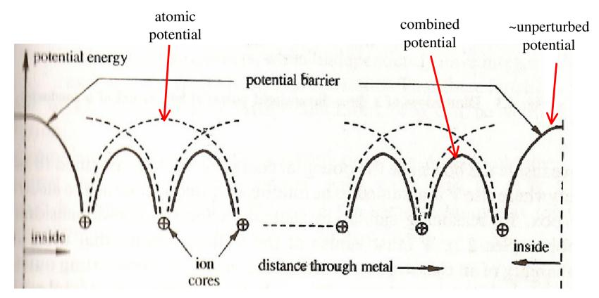
The potential barrier confines the electrons inside the faces of the conductor. Therefore we can model a conductor as unbound or free electrons confined to a potential box.
