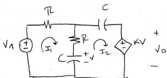
$$V_1 = RI_1 + R(I_1 - I_2) + \underbrace{\frac{1}{sc}(I_1 - I_2)}_{KV} + R(I_1 - I_2) + \frac{1}{sc}I_2 + KV = 0$$
