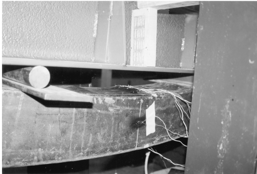
(b) Plastic Hinge and Compression Flange Local Buckling
