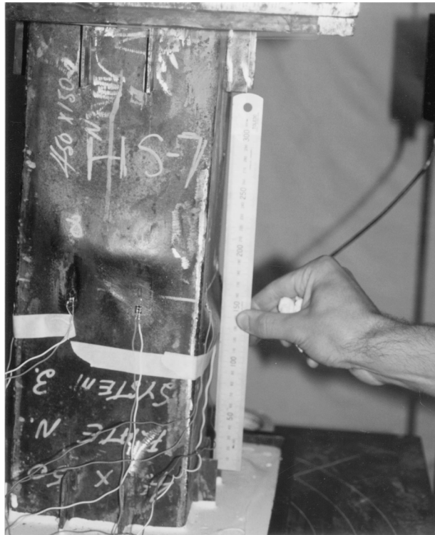
(a) Axially Loaded Column Failure
