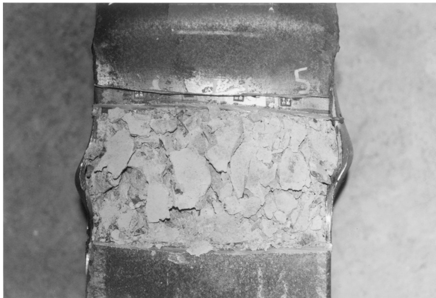
(b) Concrete Crushing
