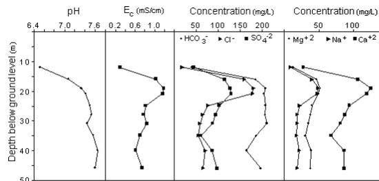
Figure 2. Depth variations in inorganic hydrochemistry derived from sampling the multi-level piezometer installed in the Triassic sandstone aquifer of north-central Nottingham.
