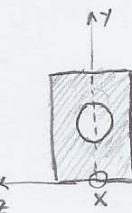
$$\Rightarrow \bar{y} = \frac{\bar{y}_1 A_1 - \bar{y}_2 A_2}{A_1 - A_2} = \frac{60.91600 - 70.2827,43}{91600 - 2827,43} \Rightarrow \boxed{\bar{y} = 55,83 \text{ [mm]}}$$
