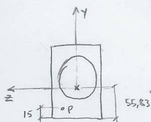
$$\Rightarrow \tau = - \frac{150.000 \text{ [kg mm].} \cdot (55,83 - 15) \text{ [mm]}}{10483044,4 \text{ [mm}^4\text{]}}$$
