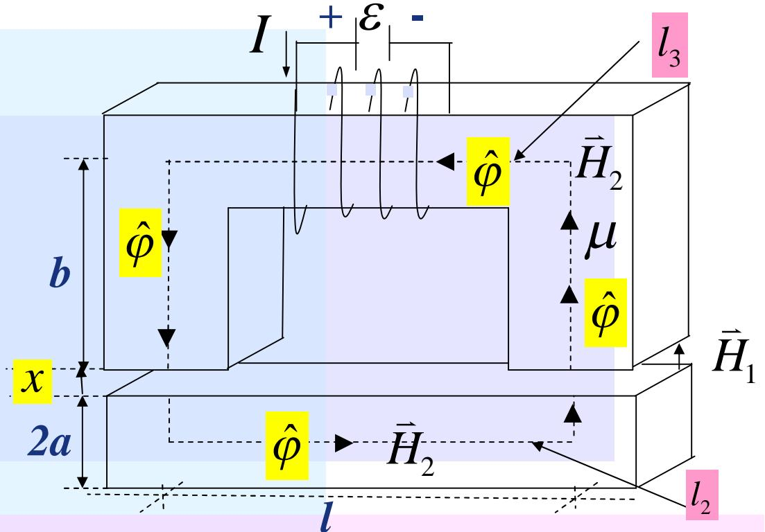
$$U = \iiint_{\Omega} \frac{1}{2} (\vec{H} \cdot \vec{B}) dv \Rightarrow U = \frac{1}{2} H_1 B_1 Vol_1 + \frac{1}{2} H_2 B_2 Vol_2$$
