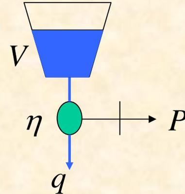
$$V_k - V_{k-1} = \Delta V [m^3] = q \left[ \frac{m^3}{s} \right] \cdot t [s]$$
