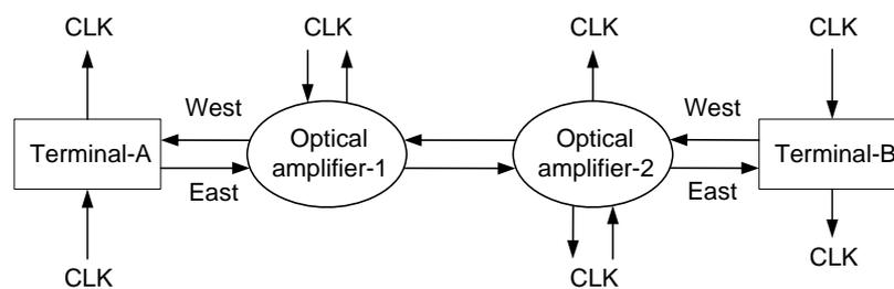
**Figure 4-7** Schematic diagram of clock transmission
