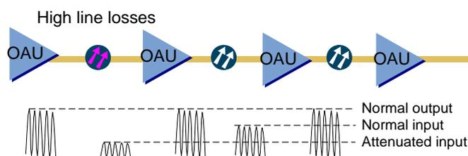
**Figure 4-3** System power when ALC is activated
