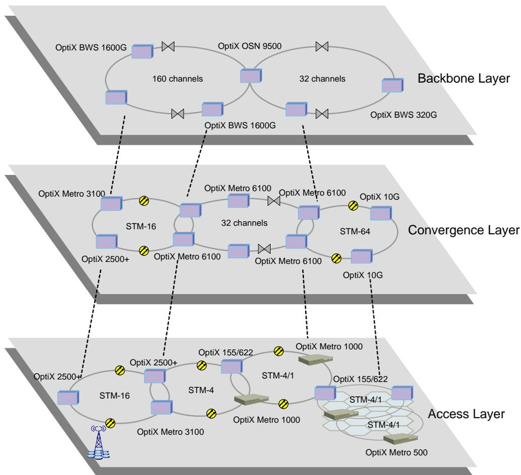
**Figure 1-1** OptiX BWS 1600G in a transmission network
