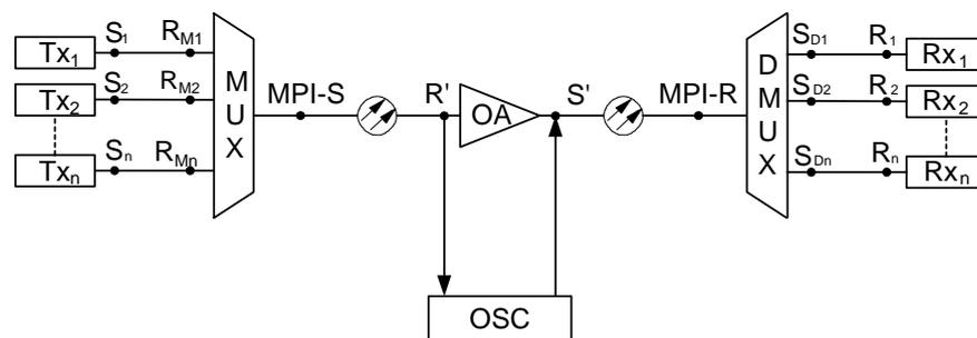
**Figure 6-1** Typical DWDM network diagram
