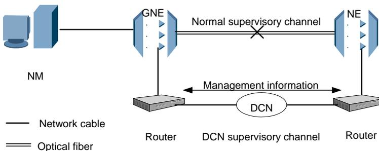
**Figure 5-14** Network management through the DCN supervisory channel
