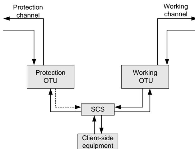
**Figure 5-5** Client-side optical channel protection
