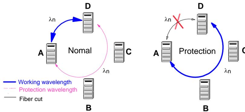
**Figure 5-3** Schematic diagram of optical channel protection
