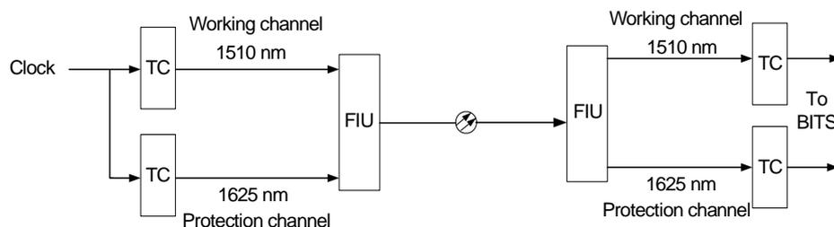
**Figure 5-8** Schematic diagram of clock channel protection (dual-fed and dual-receiving)
