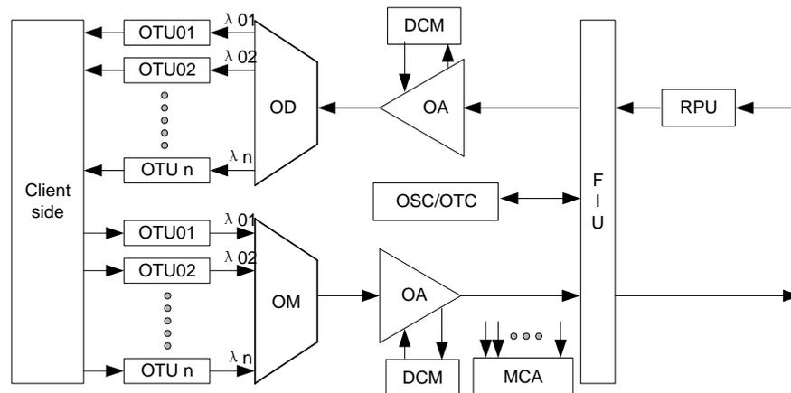
**Figure 3-1** OTM signal flow
