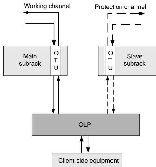
**Figure 5-6** Inter-subrack 1+1 optical channel protection
