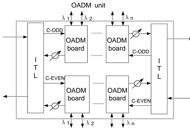
**Figure 3-17** Structure of the OADM in type I system
