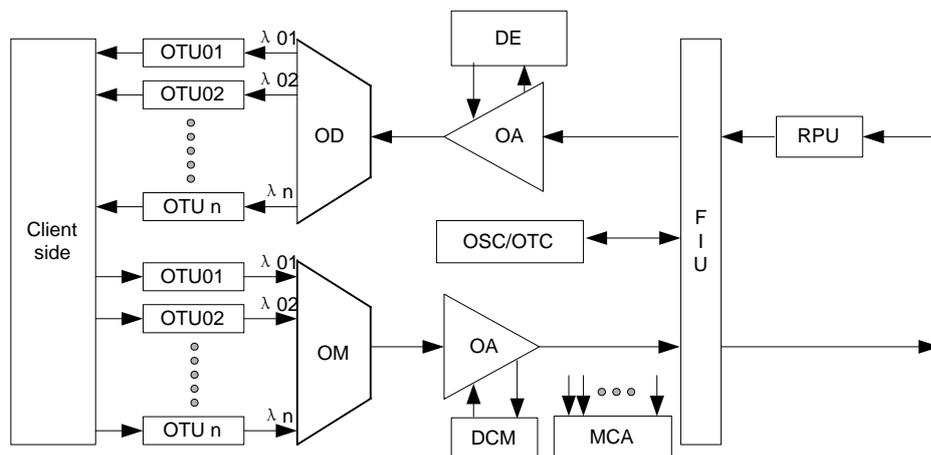
Figure 3-25 Signal flow of dispersion equaliser in OTM
