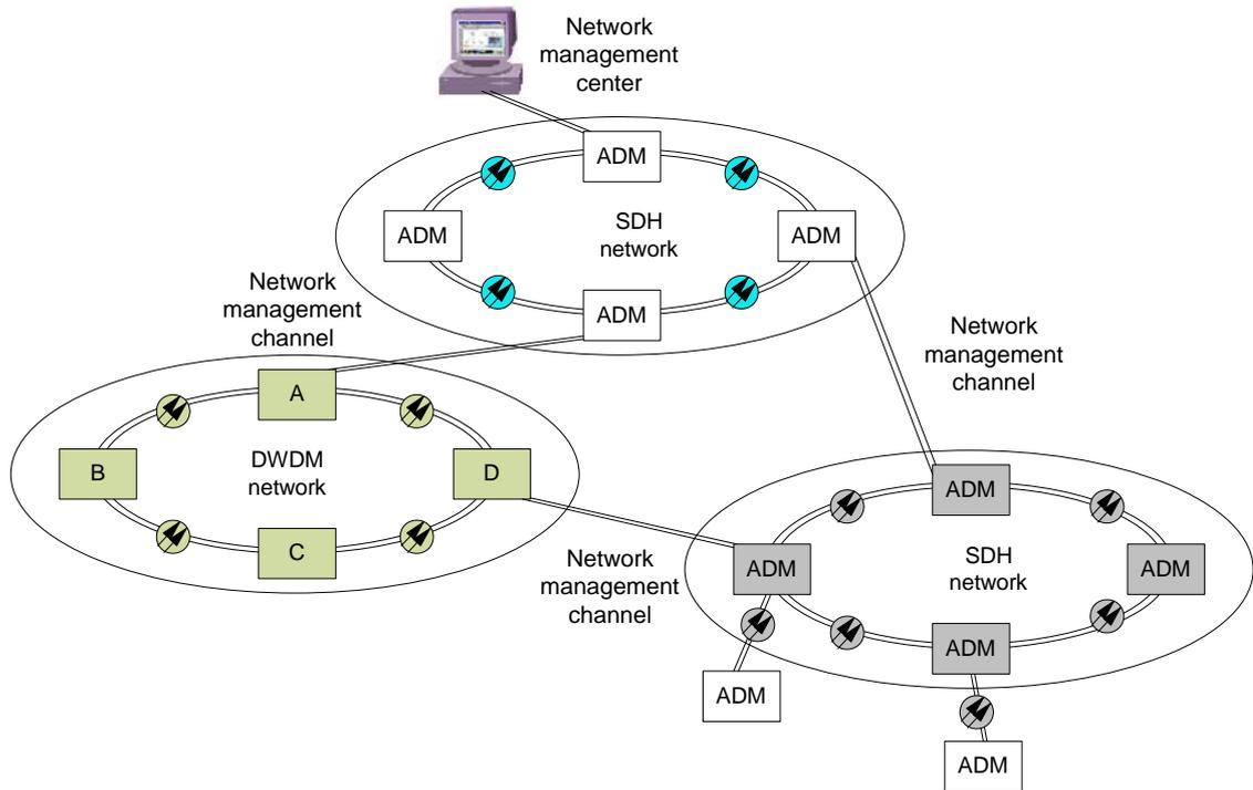
**Figure 5-15** Supervision over OptiX transmission network
