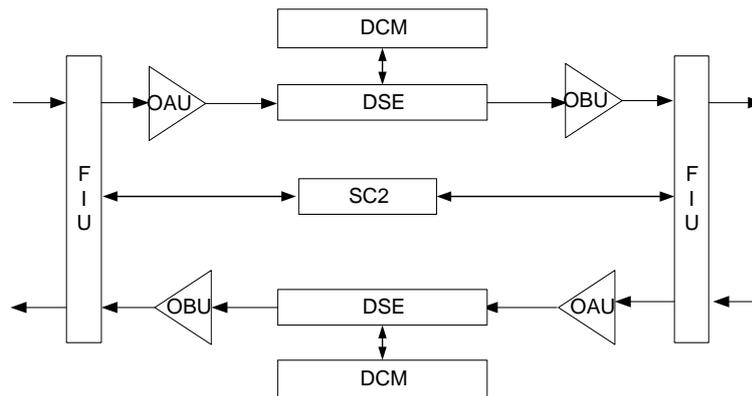
DSE: Dispersion slope equaliser unit      OAU: Optical amplifier unit
