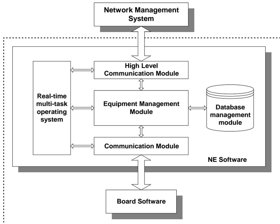
Figure 2-4 Software architecture of the OptiX BWS 1600G
