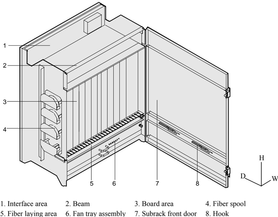
**Figure 2-1** OptiX BWS 1600G subrack
