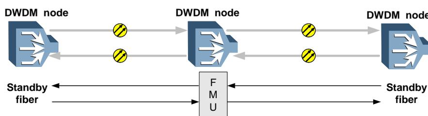
**Figure 4-11** Embedded OAMS architecture (standby fiber monitoring)
