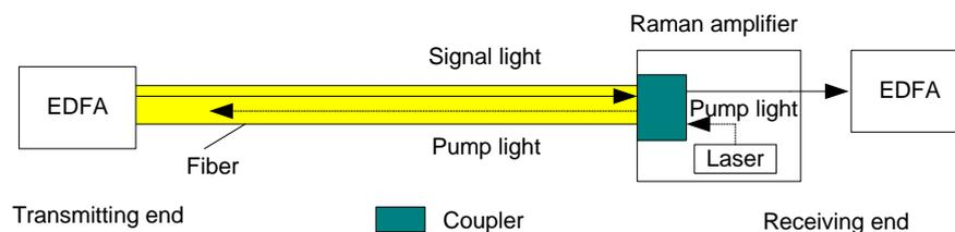
**Figure B-2** Raman amplification application in OptiX BWS 1600G system
