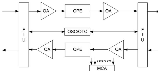
**Figure 3-23** Signal flow of optical power equaliser.
