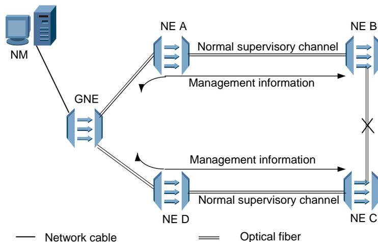
**Figure 5-12** Network management protection in ring network (a certain section fails)
