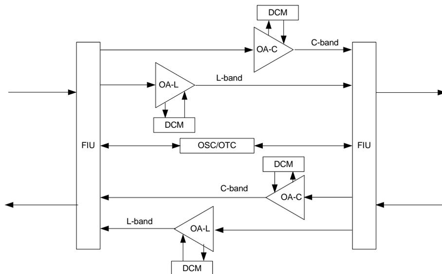
**Figure 3-11** OLA signal flow
