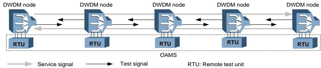
**Figure 4-9** Bidirectional test diagram
