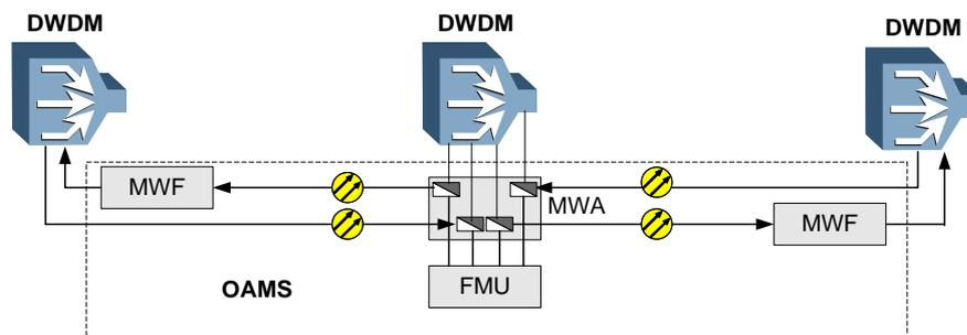
**Figure 4-10** Embedded OAMS architecture (online monitoring)
