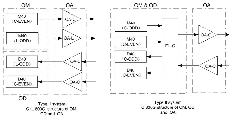
**Figure 3-3** Structure of OM, OD, OA of the type II system
