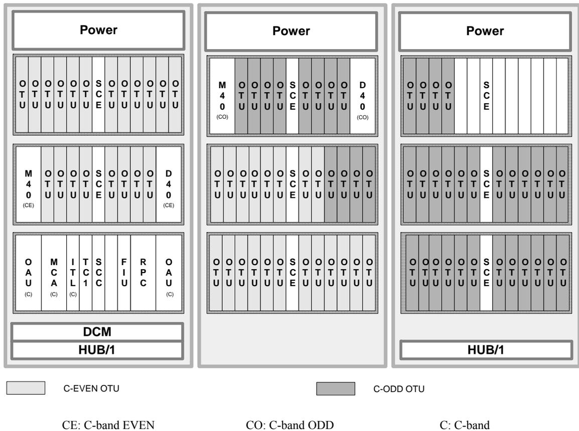
**Figure 3-8** Configuration of the C band 800 Gbit/s OTM (type II system)
