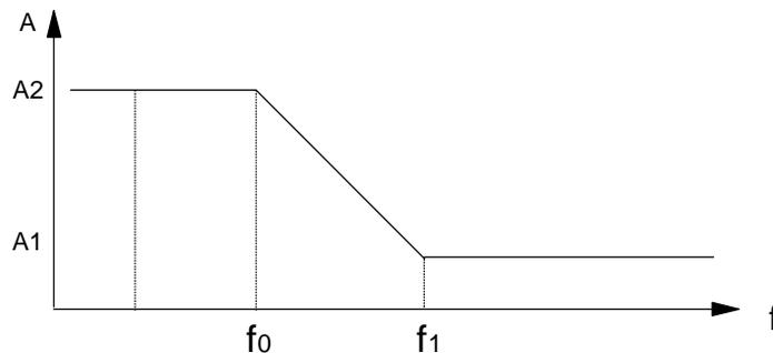
Figure 6-4 OTU input jitter tolerance
