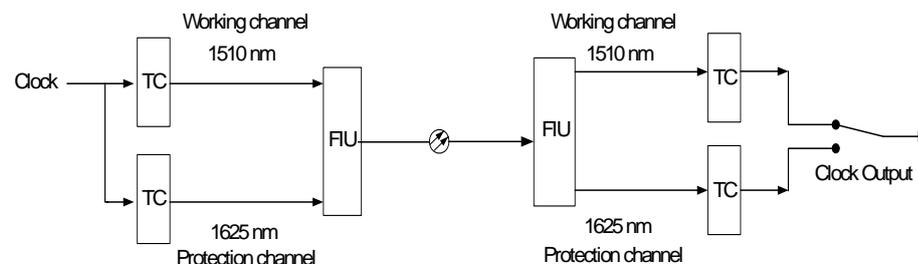
**Figure 5-9** Schematic diagram of clock channel protection (dual-fed signal selection)
