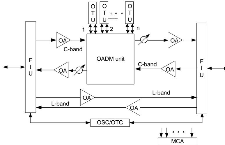
**Figure 3-14** Signal flow of the serial OADM
