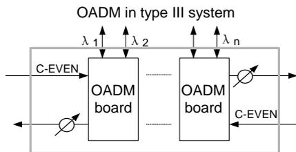
**Figure 3-19** Structure of the OADM in type III system
