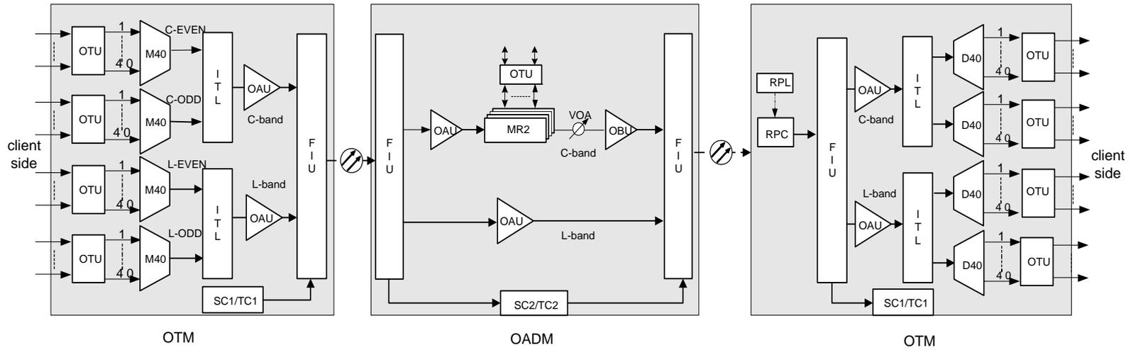
**Figure 2-2** Positions of the boards in the system
