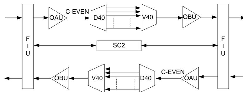
V40: 40-channel multiplexing unit with VOA
