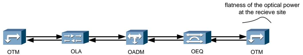
**Figure 4-4** Flatness of the optical power at the receive end when APE is not activate
