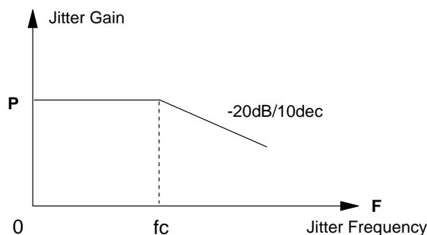
**Figure 6-2** OTU jitter transfer characteristics
