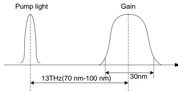
**Figure B-1** Raman amplifier gain spectrum
