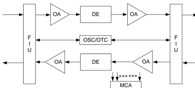
**Figure 3-24** The signal flow of dispersion equaliser
