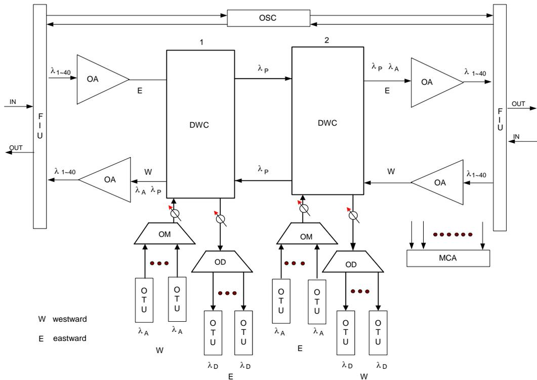
**Figure 3-16** Signal flow of the ROADM
