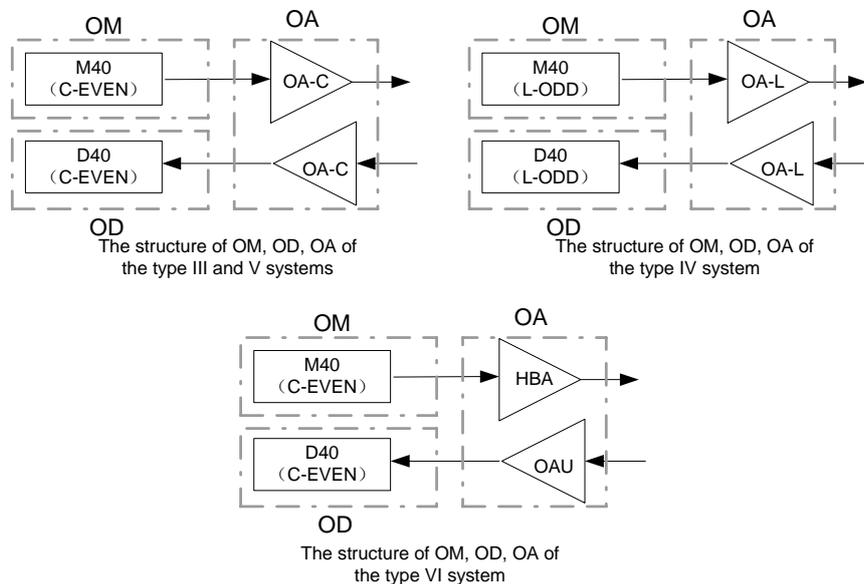
**Figure 3-4** Structure of OM, OD, OA of the type III, IV, V and VI systems
