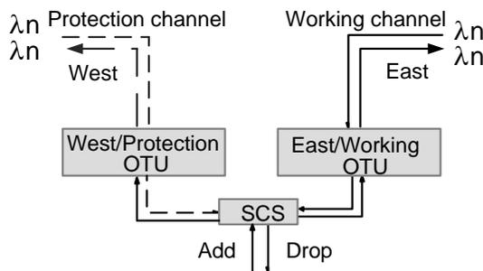
**Figure 5-4** Inter-OTU 1+1 optical channel protection
