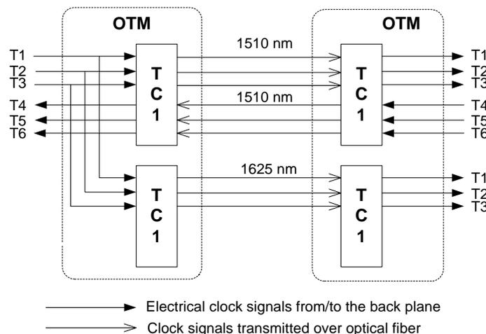
**Figure 5-10** Configuration of the system with clock protection function but without add/drop of clock signals at intermediate stations
