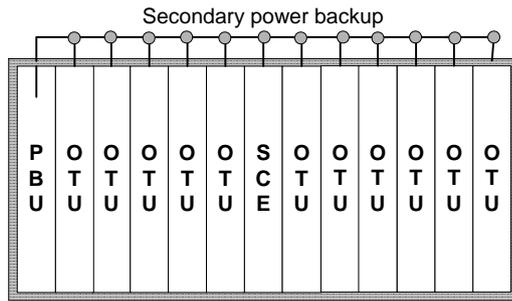
**Figure 5-1** Centralised power protection for OTUs
