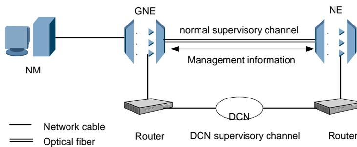
**Figure 5-13** Network management through the normal supervisory channel
