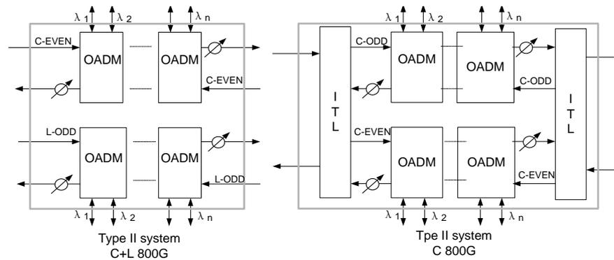
**Figure 3-18** Structure of the OADM in type II system
