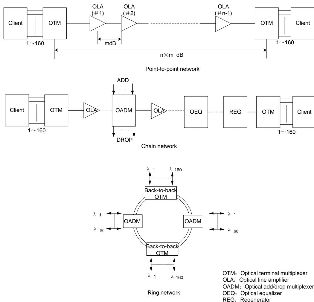
**Figure 4-1** OptiX BWS 1600G networking diagram
