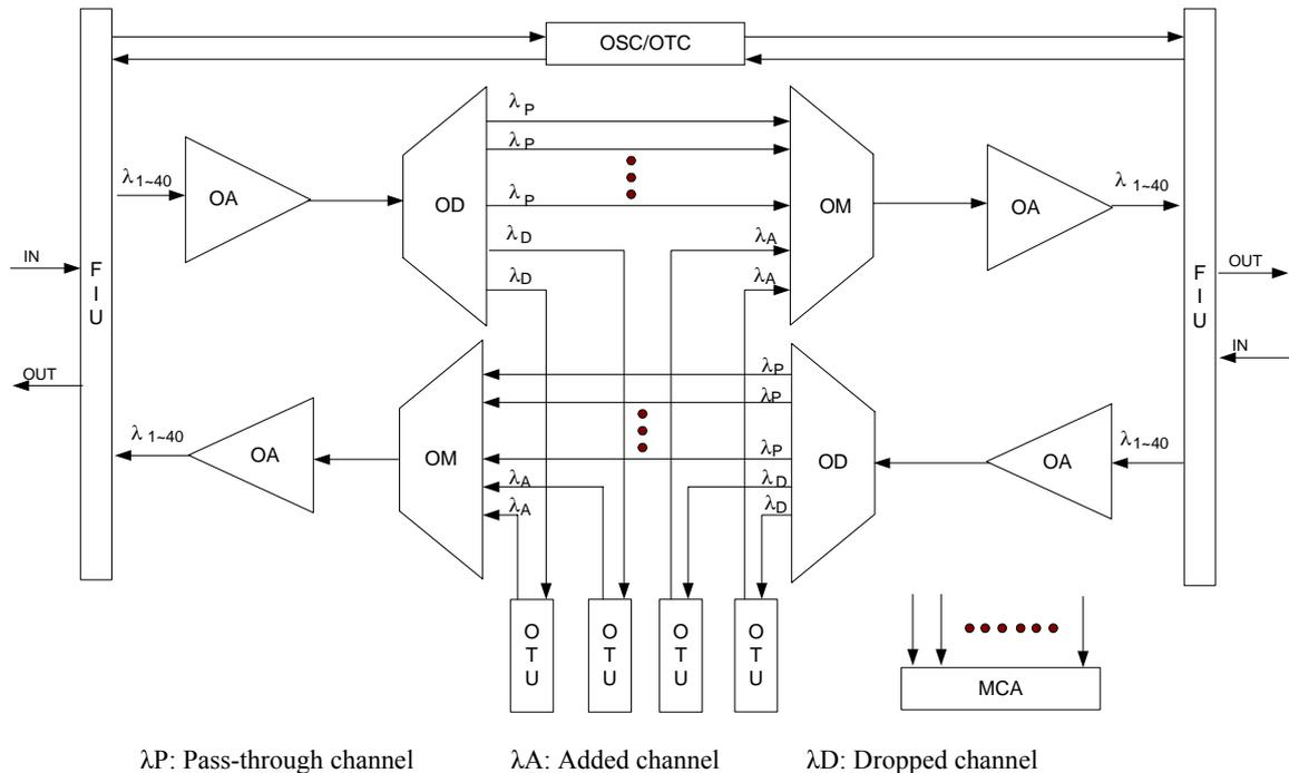
**Figure 3-15** Signal flow of the parallel OADM
