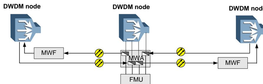
**Figure 2-3** Structure of the embedded OAMS application (online monitoring)
