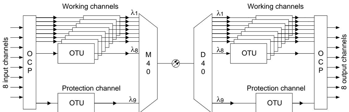
**Figure 5-7** Schematic diagram of 1:N (N≤8) OTU protection
