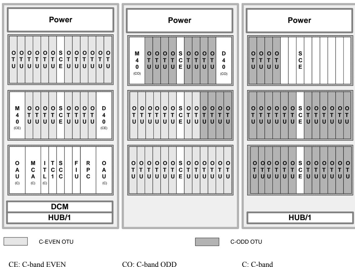
**Figure 3-5** Configuration of the C-band 800 Gbit/s OTM (type I system)
