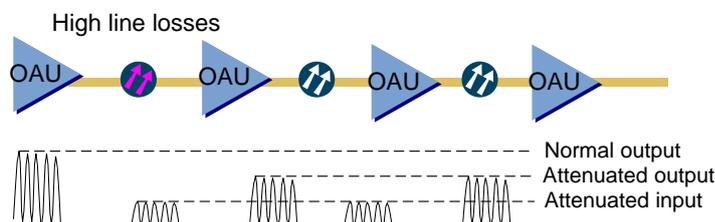
**Figure 4-2** System power when ALC is not activated
