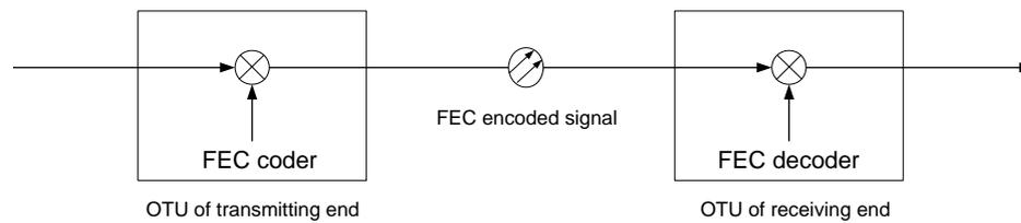
Figure 6-3 OTU with out-band FEC function
