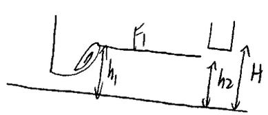
$\Delta X = L - L_r; \Delta X = \frac{E_1 - E_2}{\bar{J} - i}; L_r = 10,2 \text{ [m]}$
