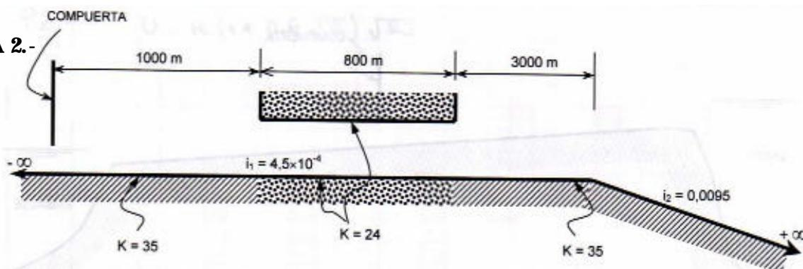
Altura crítica:  $h_c = \left(\frac{q^2}{g}\right)^{1/3} = \left(\frac{1}{g} \left(\frac{Q}{b}\right)^2\right)^{1/3} = \left(\frac{3,5^2}{9,8}\right)^{1/3}$
