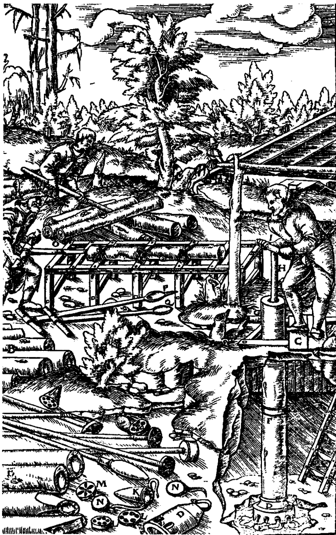
Fig. 3. Manually operated single-action piston pump with details of rods, pipe drilling, flapper valves, and leather gaskets
