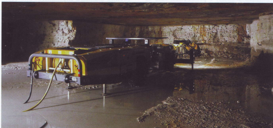
Rocket Boomer S1 L drilling in low headroom.
