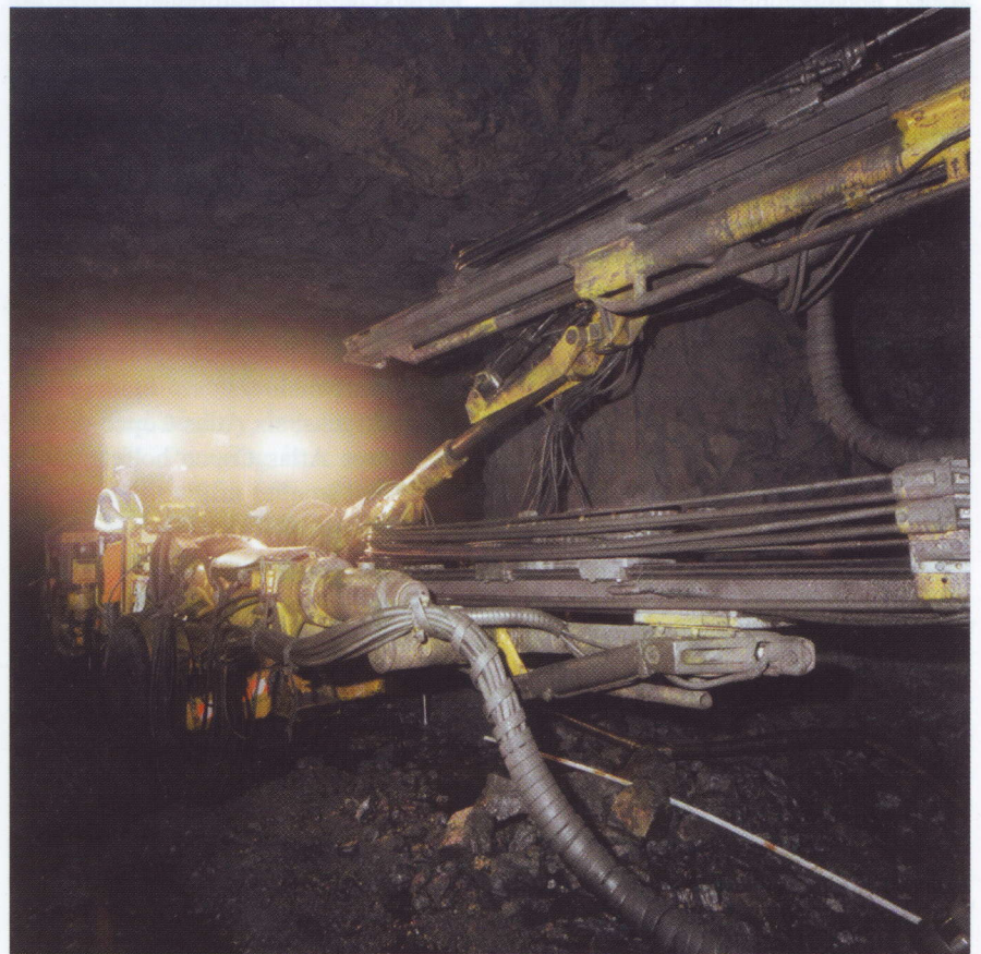
Atlas Copco Rocket Boomer 322 mounted with COP 1238ME rockdrill at a production face.
