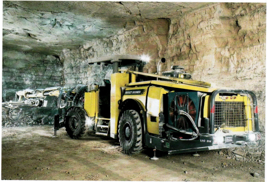
Atlas Copco Rocket Boomer L1C-DH drilling the face at Auersmacher limestone mine.
