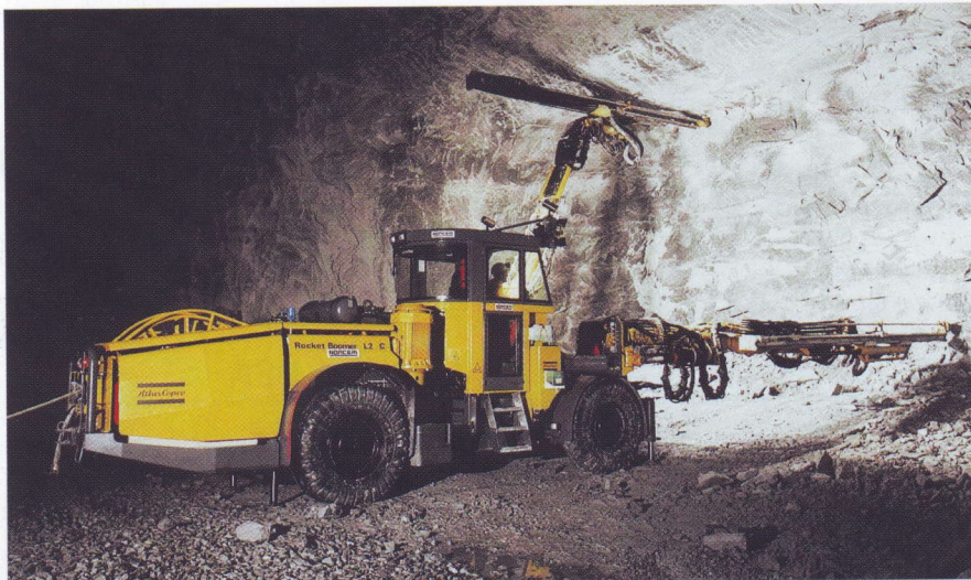
Norcem Rocket Boomer L2 C drilling a top heading at Dalen mine.
