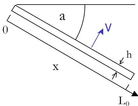
$$\begin{aligned} dM &= \Delta \mathbf{r} \cdot gh \cos(a)(L_0 - x)dx \Rightarrow \\ M(x) &= -\frac{1}{2}\Delta \mathbf{r} \cdot gh \cos(a)(L_0 - x)^2 \\ V(x) &= \frac{dM}{dx}(x) = \Delta \mathbf{r} \cdot gh \cos(a)(L_0 - x) \\ \frac{d^2 \mathbf{w}}{dx^2}(x) &= \frac{-M(x=0)}{D}; \frac{d^3 \mathbf{w}}{dx^3}(x) = \frac{-V(x=0)}{D} \end{aligned}$$
