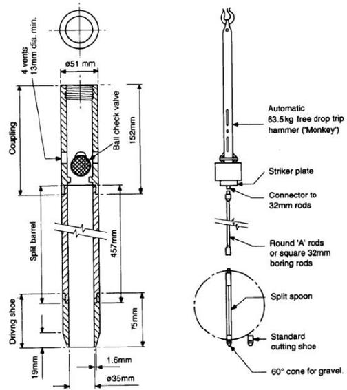
Fig. 9.1 Equipment for the standard penetration test.
