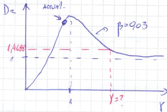
$$\Rightarrow \frac{\gamma^2}{\sqrt{(1-\gamma^2)^2 + (2p\gamma)^2}} = 1,4688 \Rightarrow \gamma = 1,7688$$
