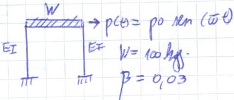
$\bar{\omega} = 12 \text{ rad/seg.} \Rightarrow \bar{T} = 0,5236 \text{ seg}$
