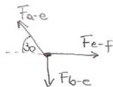
$$\begin{aligned}\sum F_x = 0 &\Rightarrow F_{e-f} - F_{a-e} \cdot \cos 30^\circ = 0 \\ \sum F_y = 0 &\Rightarrow F_{a-e} \cdot \sin 30^\circ - F_{b-e} = 0\end{aligned}$$
