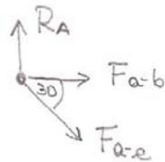
$$\begin{aligned}\sum F_x = 0 &\Rightarrow F_{a-b} + F_{a-e} \cdot \cos 30^\circ = 0 \\ \sum F_y = 0 &\Rightarrow R_A - F_{a-e} \cdot \sin 30^\circ = 0\end{aligned}$$
