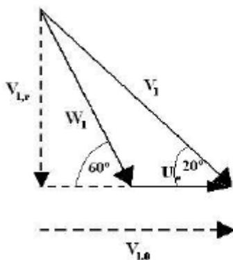
$$1) \quad V_{1,t} = V_1 \cdot \text{sen}(20^\circ) = W_1 \cdot \text{sen}(60^\circ)$$
