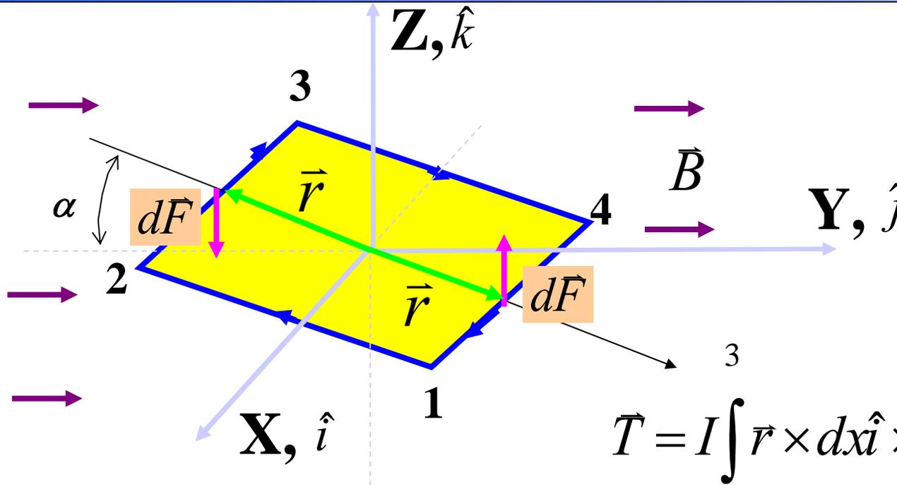
$$\vec{T} = I \int_2^3 \vec{r} \times d\vec{x} \hat{i} \times \vec{B} + I \int_4^1 \vec{r} \times d\vec{x} \hat{i} \times \vec{B}$$
