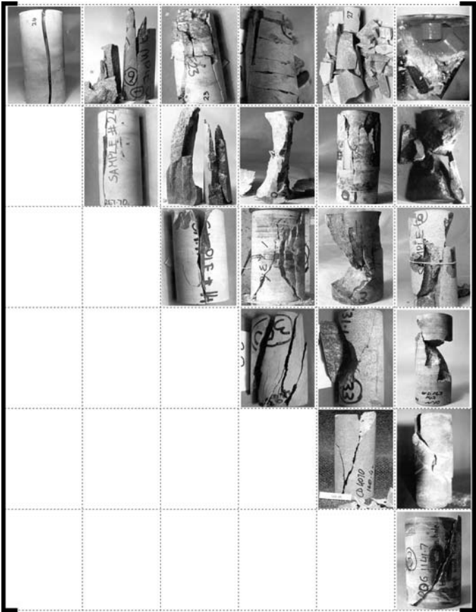
Fig. 4. A matrix form of failure modes of rock samples tested in uniaxial compression
