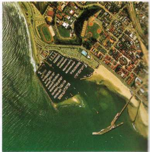
(B) The initial breakwater prevented the generation of longshore currents in the protected area behind it, and therefore the harbor filled with sand.
