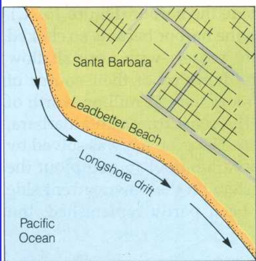
(A) The Santa Barbara coast had significant longshore drift before the breakwater was built.
