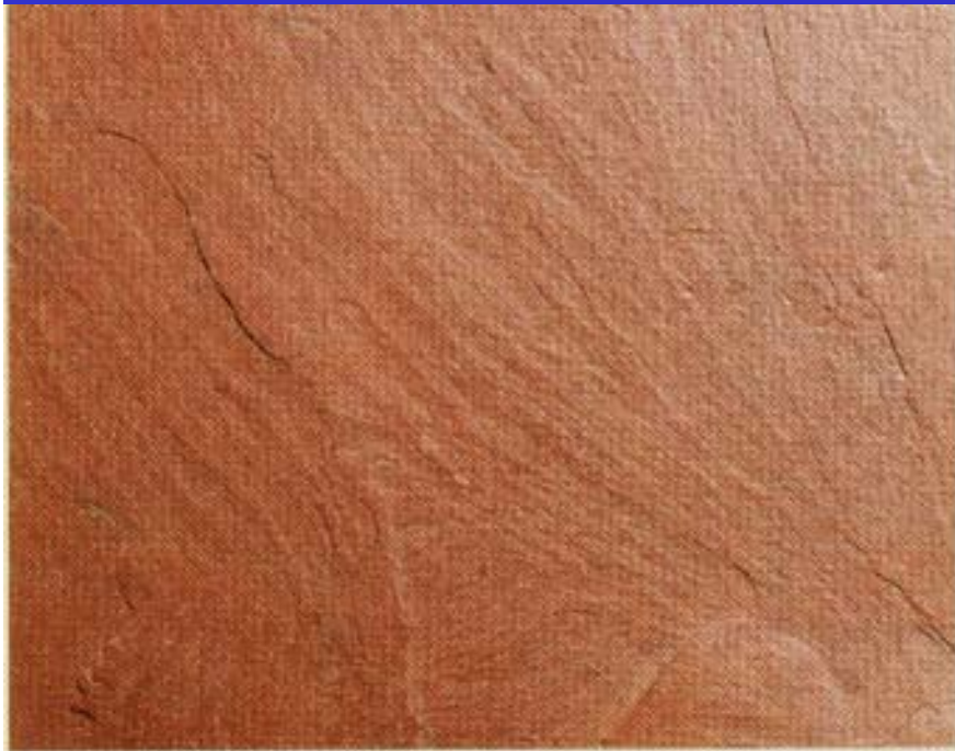
(A) Slate is a fine-grained foliated rock. The foliation usually cuts across sedimentary bedding.
