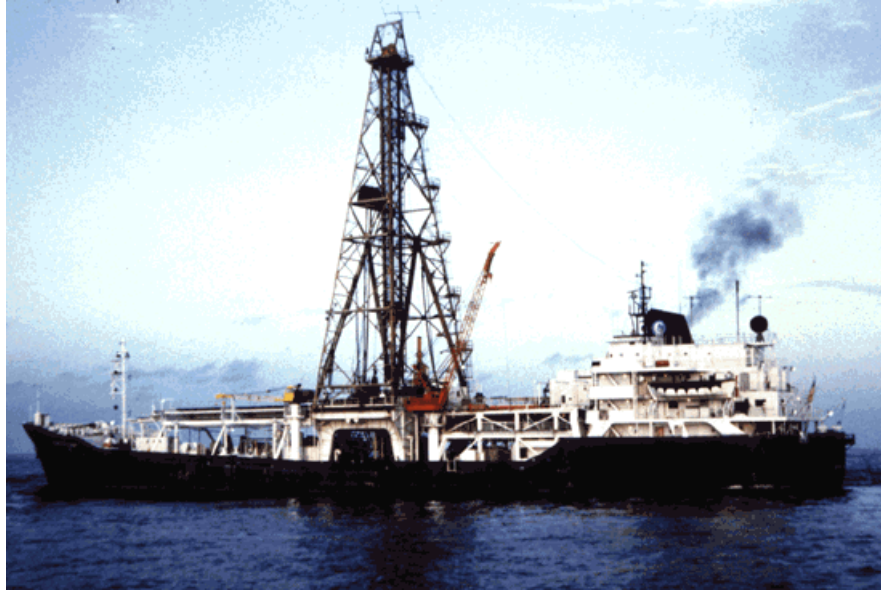
Above: The Glomar Challenger was the first research vessel specifically designed in the late 1960s for the purpose of drilling into and taking core samples from the deep ocean floor. Below: The JOIDES Resolution is the deep-sea drilling ship of the 1990s (JOIDES= J oint O ceanographic I nstitutions for D eep E arth S ampling). This ship, which carries more than 9,000 m of drill pipe, is capable of more precise positioning and deeper drilling than the Glomar Challenger. (Photographs courtesy of Ocean Drilling Program, Texas A & M University.)
