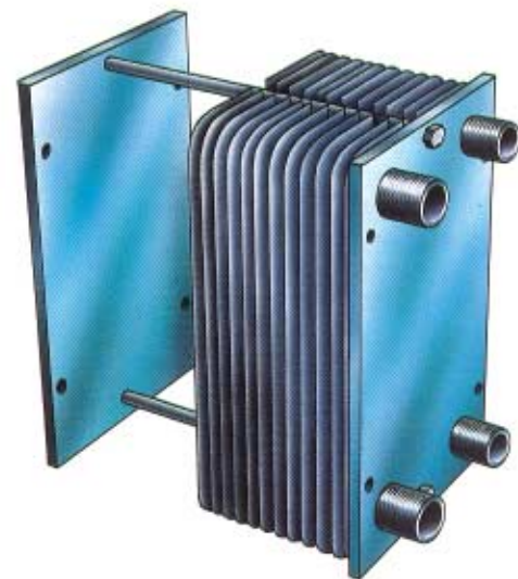
3. Then the plates corresponding to the plate specification are positioned in the frame.
