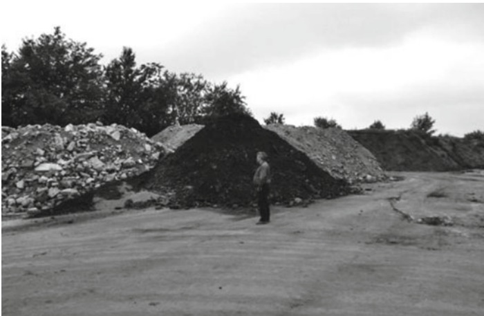
Fig. 6.18 Different substrates deposited before the biological treatment occurs in a remediation plant (With kind permission of DHC company, Freiberg, Germany)
