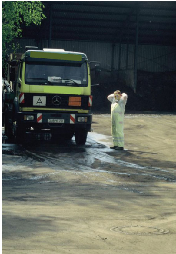
Fig. 4.3 Truck-wash plant operated by a worker wearing protective clothes and breather
