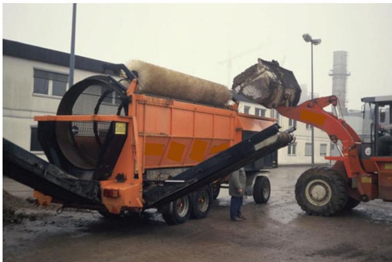
Fig. 4.12 Process of soil mixing for the supply of clean soil: drum-sieve for mixing as well as for organic matter addition purposes
