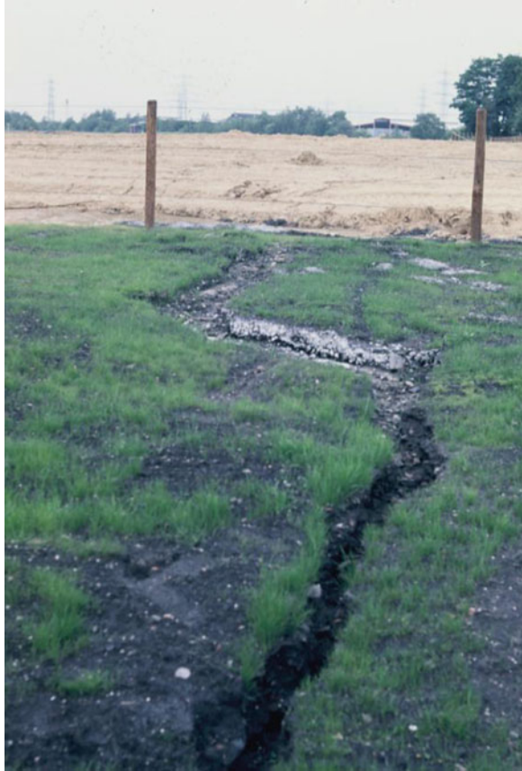
Fig. 6.26 Deposit of decontaminated soil obtained from the thermal treatment (pyrolysis) in Essen, Germany; gully erosion in spite of a low slope gradient and salt crust formation ( white colour ) are visible
