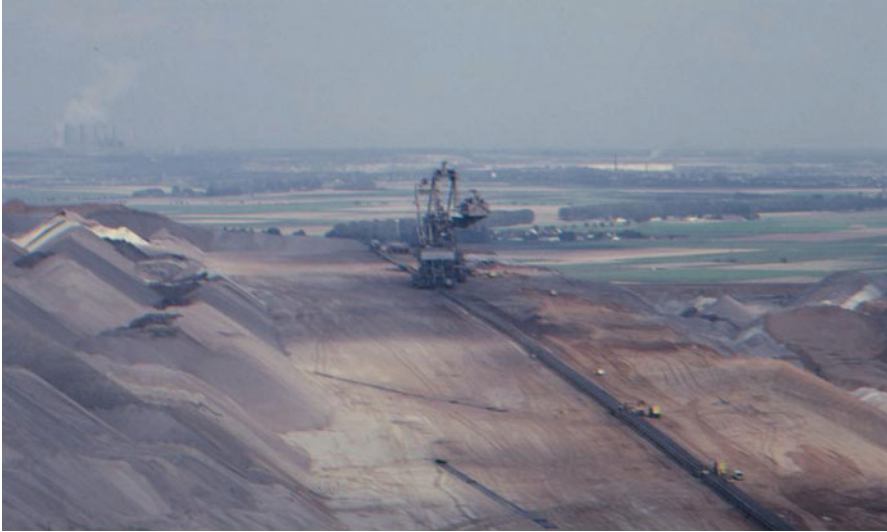
Fig. 3.2 Different overburden deposited by belt stackers in the Rhineland lignite coal open-cast mining area, Germany
