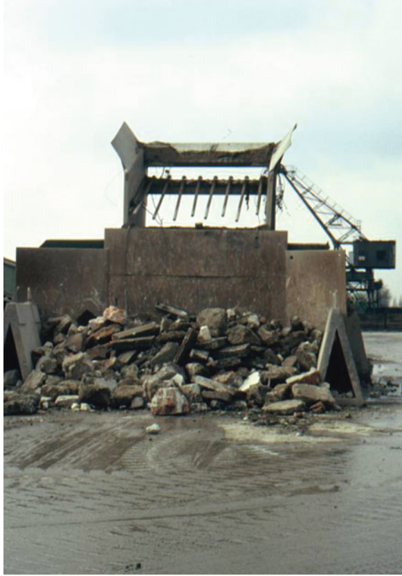
Fig. 6.2 Grizzly device to separate construction debris, masonry and bulky refuse
