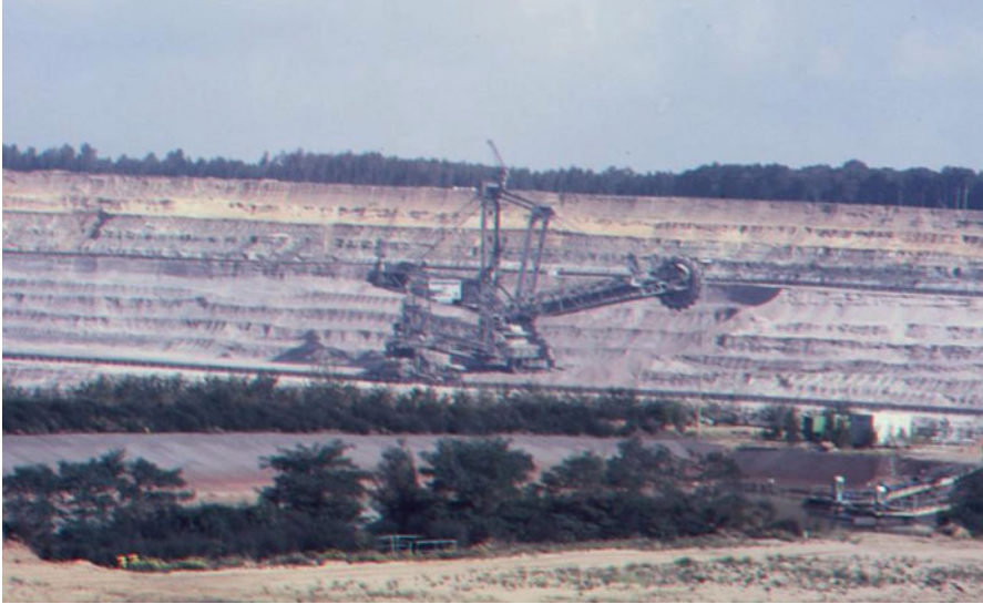
Fig. 3.1 Bucket wheel excavator in the Rhineland lignite coal open-cast mining area, Germany
