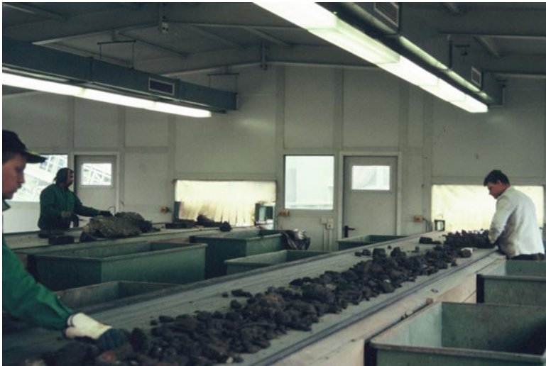
Fig. 6.4 In-door picture of the small housing for removal of waste components; workers are busy collecting large waste materials transported on a conveyor belt
