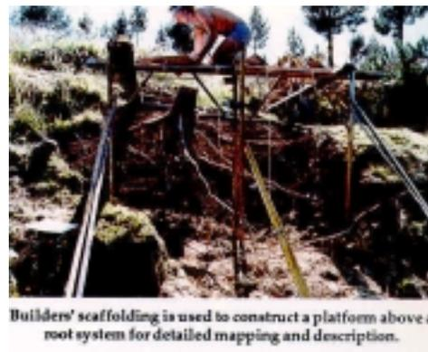
Builders' scaffolding is used to construct a platform above a root system for detailed mapping and description.
