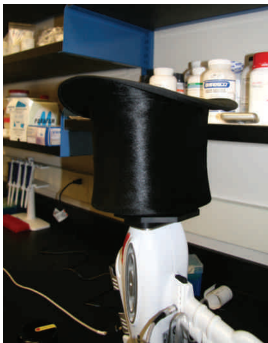
▲ 5. Late 19th-century fur felt hat (above) from the collection of the Bata Shoe Museum being tested (below) by being placed on a portable XRF machine in Professor Ana Pejović-Milić's physics lab. Test performed by Eric Da Silva, Ryerson University. It contained trace amounts of mercury. Top: E. Baumann and Sohne Hutmacher, Switzerland. Copyright © 2015 Bata Shoe Museum, Toronto (Photo: Ron Wood).
