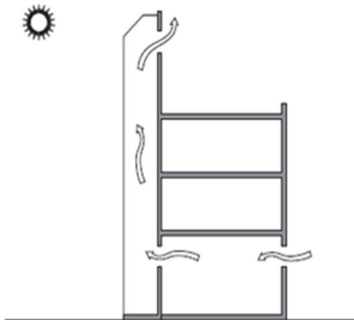
Stack ventilation using a solar chimney
