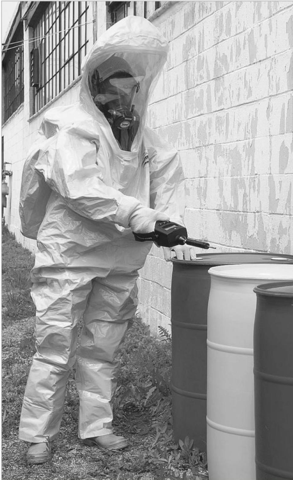
Specially designed equipment, such as chemical-resistant suits, gloves, and boots, reduce or eliminate risks related to hazardous chemical exposure.
