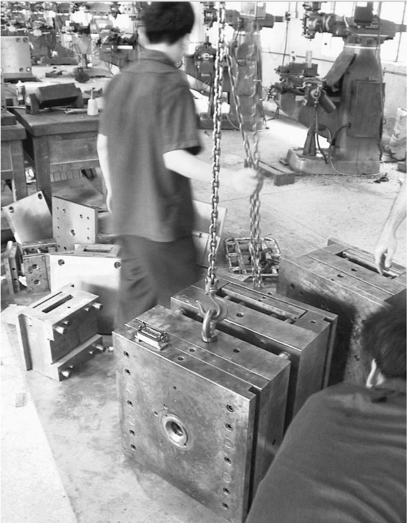
The tool is a separate module that fits into an injection-molding machine. This image shows an in-progress tool in the tooling shop.
