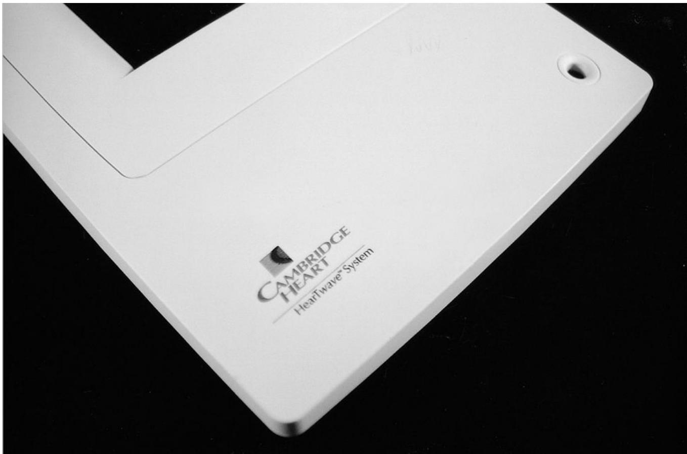
**Pad printing** is a process for printing graphics on a complex surface. Pad printing involves transferring ink from a printing plate etched with the desired image to the part by way of a silicone pad. Because the silicone pad is flexible, it can conform to the contour of the part printed without distorting the image. Extremely fine detail and tight multicolor registration are achievable. Almost any material can be pad printed, so long as compatible ink is used.
