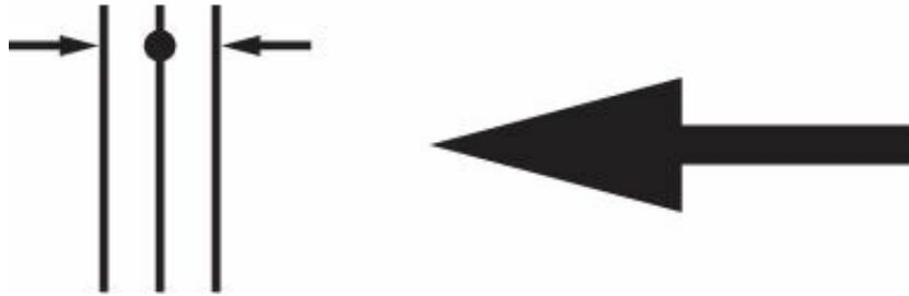
Arrow-heads are used to terminate dimension lines. Its length is about three times the depth and the space should be filled in. Adjacent arrow-heads may be replaced by clearly marked dots where space is limited.
