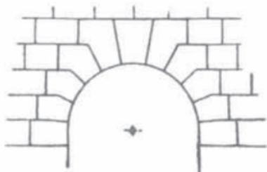
Fig. 135. ARCO APAREJADO CON DOVELAS A MONTACABALLO
