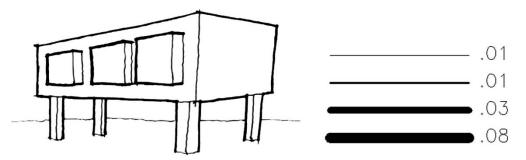
SKETCH LINE WEIGHTS: Varying line weights (thicknesses) makes sketches more dynamic, cleans them up and helps better communicate surface transitions. Use these rules and tips to tighten up your sketches.
