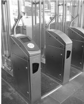
The ticket portal (Figure 20) is placed at the entrance of the station; the portal opens only when a ticket has been inserted, and hence obstructs fare dodgers' movements. The only way to fare dodge is to jump over the
