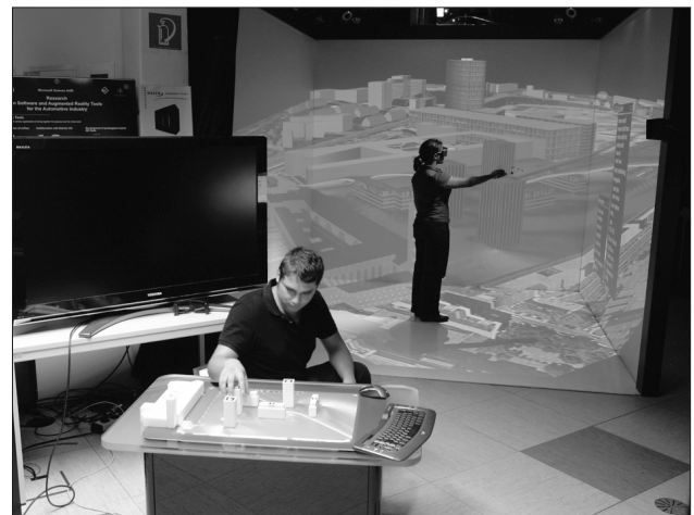
Figure b: Urban simulation of Stuttgart 21 project - visualization overlaid with the near real time simulation of air flow
