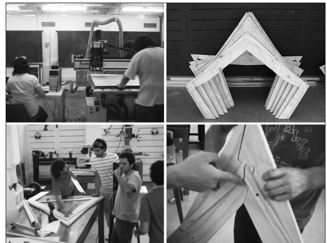
Figure 2. CNC fabrication of 890 differentiated components
