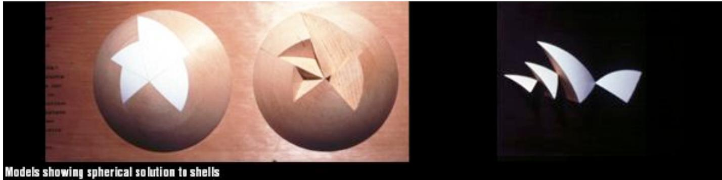
Models showing spherical solution to shells
