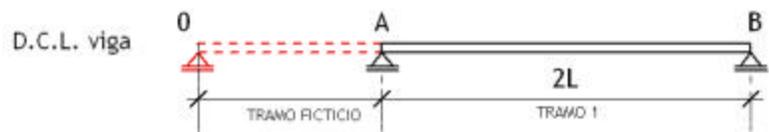
$$M_0 L_0 + 2M_A(L_0 + L_1) + M_B L_1 = 6 * [T_{c0} + T_{c1}]$$
