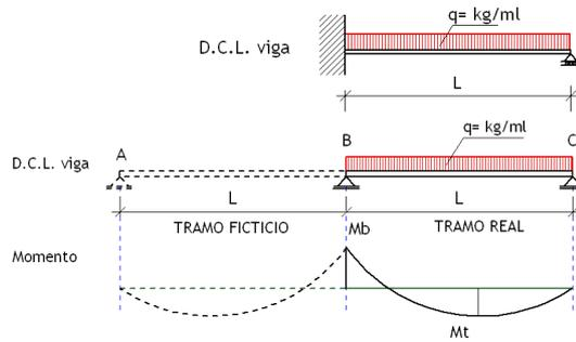
$$M_A L_1 + 2M_B (L_1 + L_2) + M_C L_2 = 6 * [T_{C_1} + T_{C_2}]$$
