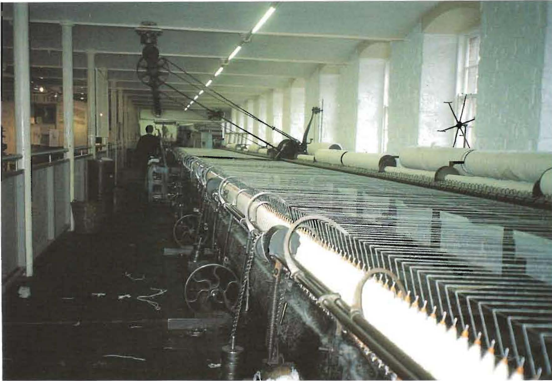
Mill Number Three, New Lanark, with Platt Brothers mule of 1891 under a brick arched, iron-framed ceiling.
